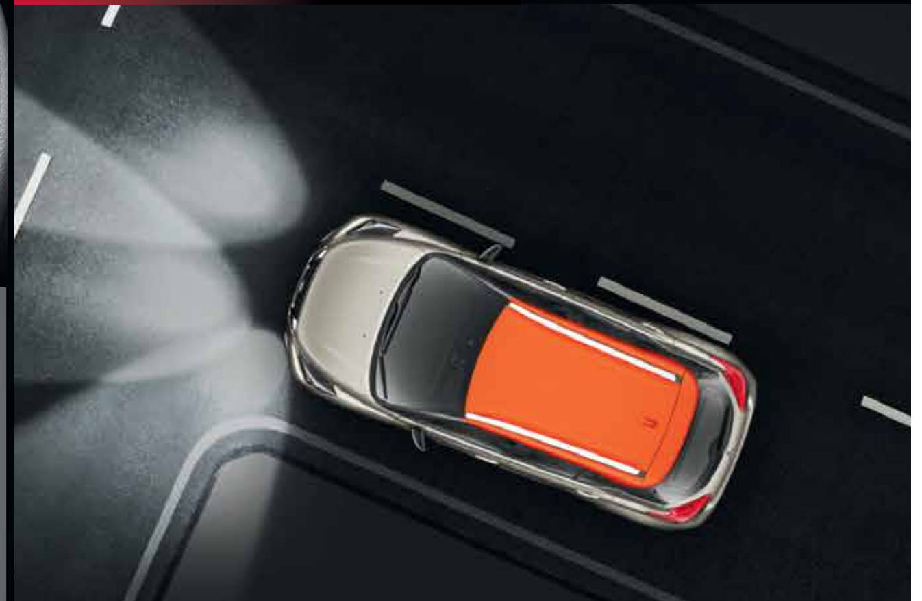
CORNERING FRONT FOG LAMPS (FOR ADDITIONAL VISIBILITY WHILE TAKING A TURN)
